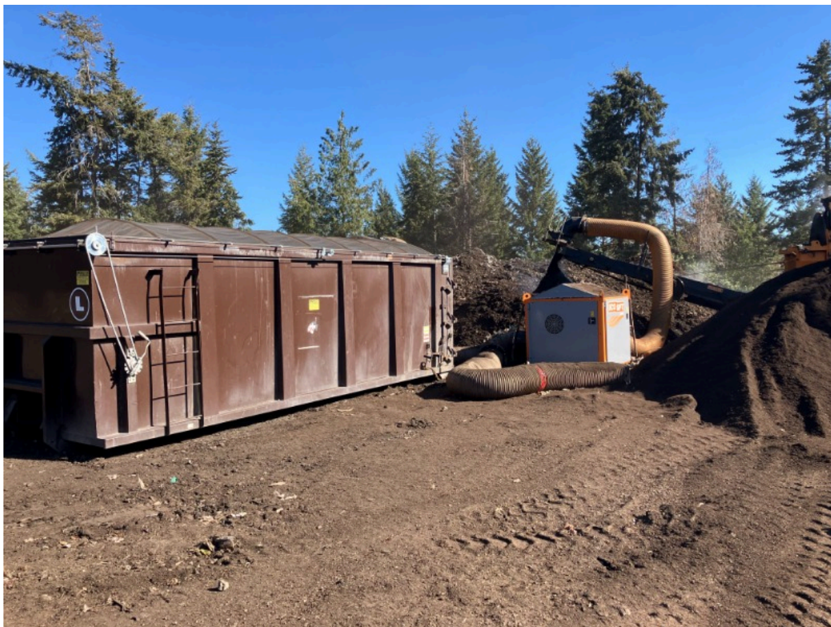
Photo 5. Residuals stored in a 15 cubic metre container, in a manner that prevents vector attraction.
